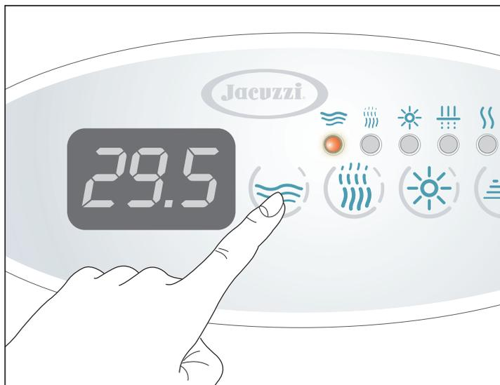
► Press the key “Pump”
