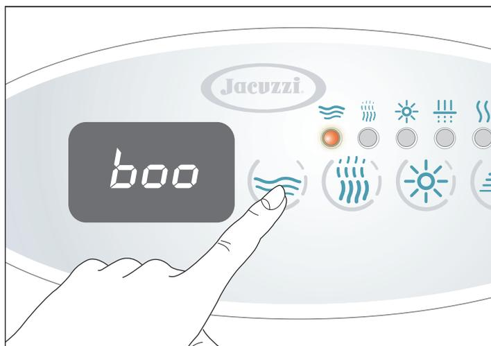
► To activate this function, press and hold down the "Pump"
