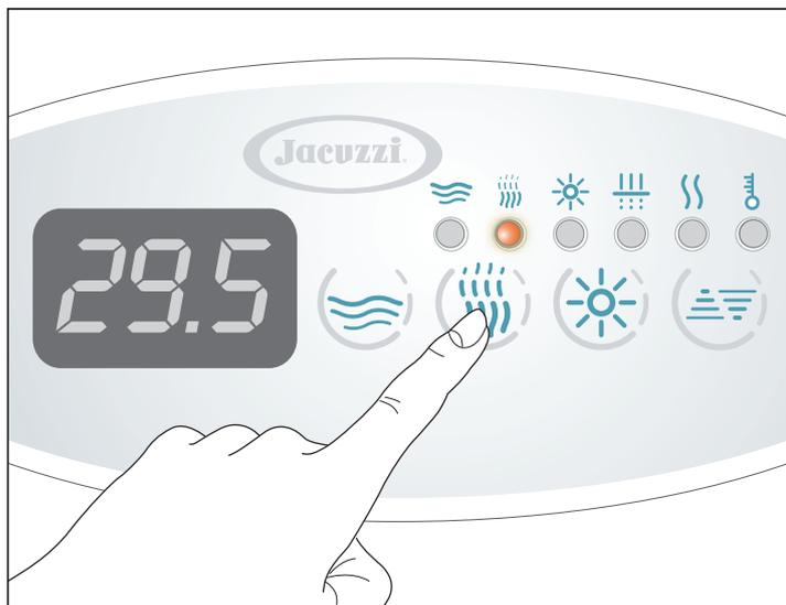
► Press the key "Blower" (🌀) to activate the air compressor (the LED comes on).
