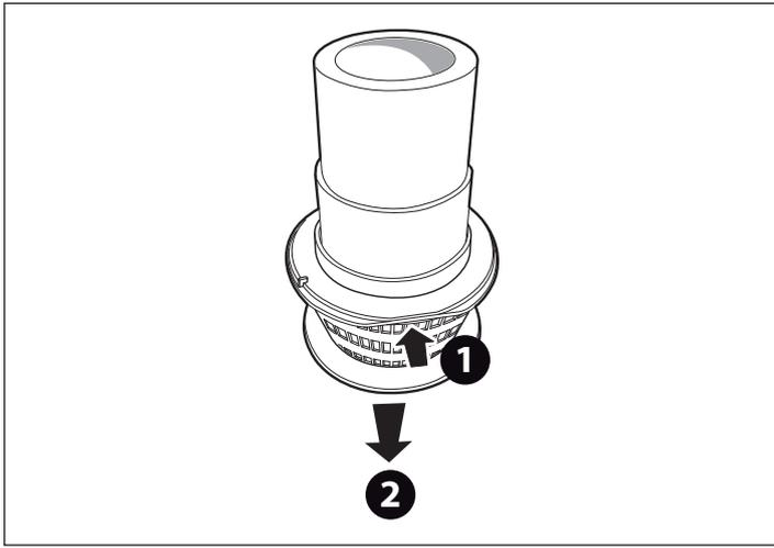
► When carrying out scheduled maintenance, if it is necessary to disassemble the skimmer basket, apply pressure to the relevant area in order to unhook the vessel; therefore disassemble it pushing downwards.
